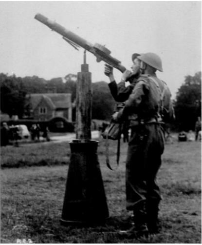
Rowland's Castle Home Guard show how an old milk churn can be used as a tripod for a light Aak-Ack (Anti-aircraft) gun to deal with low-flying enemy aircraft.
